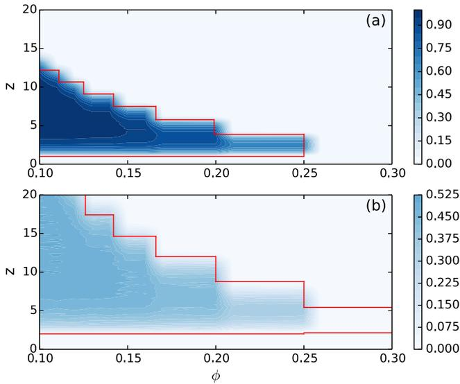
FIG. 2. Frequency  $F_g$  of global cascades as a function of node threshold  $\phi$  and average degree  $z$  for different values of  $f$ : (a)  $f = 0$ , corresponding to the original threshold model, and (b)  $f = 0.5$ . The red lines show the boundary of the global cascade regime according to Eq. (7). Simulations correspond to an ER network with size  $N = 5000$  and are averaged over  $10^4$  realizations.
