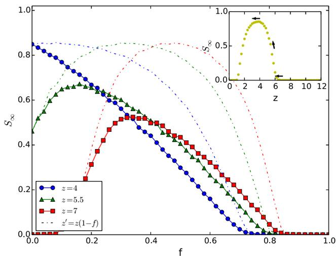
FIG. 3. Final average cascade size  $S_\infty$  as a function of  $f$  for different values of average degree  $z$ , compared with the results on ER networks with average degree  $z' = z(1 - f)$  (dashed lines). The inset shows how  $S_\infty$  changes with  $z$  in the original Watts model. The parameters in the simulations are  $N = 5000$  and  $\phi = 0.18$ . All results are averaged over  $10^4$  realizations.
